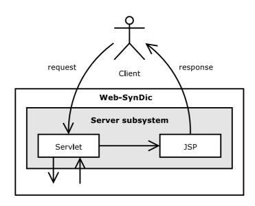
The next UML diagram was produced at the design stage of the project and represents the architecture of the Server subsystem.
